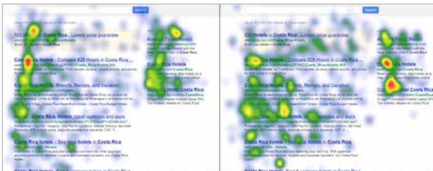
Figure 3. Gaze distribution heatmap laid over 2D (to the left) and 3D (to the right) web search engine results page as seen in ( González-Zúñiga et al., 2013 ). Please note, in the 3D stimulus the block with advertising (to the right) is placed closer to the user in the stereo space resulting in higher concentration of the observers' attention
